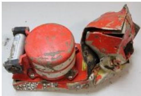
Photo 2 Damaged CVR of crashed A320 (Origin: ditto)
